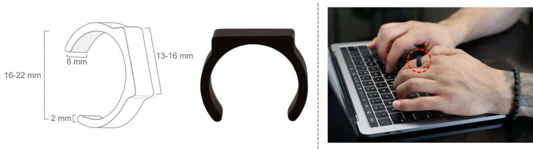
Fig. 2. (Left) Design, specifications, and model of the ring used within the study. The mock smartring has a 2mm thick and 6mm wide loop. The diameters used for our mock smartrings were created between 16mm and 22mm and constructed in intervals of 0.5mm. The length of the top surface increases accordingly, from 13mm to 16mm, with larger diameters of the ring. (Right) An example of a participant wearing the mock smartring during their daily life.
