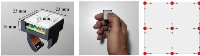
**Figure 1: Left: Dimensions of the smart-ring; Middle: Scale relative to the hand while wearing the smart-ring; Right: The 9 touch surface locations and the corresponding 24 directions explored in the study.**
