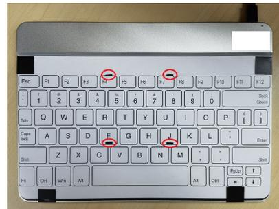
Figure 3: The Sensel Morph used, with the printed layout attached for all studies. Highlighted with red ovals are the locations of the physical markers (used only when collecting resting data in Section 4.1) placed on the “f” and “j” keys as well as near the top of the force sensor.
