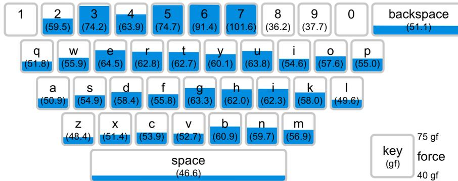
**Figure 1: Mean maximum forces applied to keys across participants, captured from a three-state, force sensitive, virtual keyboard while 10-finger typing. Our analysis shows that using a force threshold function (i.e., T-Force) allows us to propose methods for classifying touch events between keypresses and non-keypresses. Furthermore, accommodating the variations seen, we can further improve the utilization of force in classification.**
