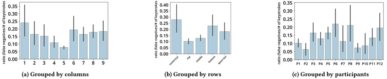
Figure 10: False negatives as a ratio between the false negatives and the total number of keystrokes detected across dimensions during the user study with the three-state keyboard with a constant force threshold. Black lines denote 95% confidence intervals.
